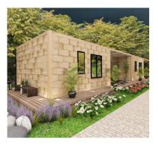
The Bio-Bricks can be used for the construction of green buildings everywhere, independently from climate characteristics of the environment as the Bio-Bricks are able to naturally manage the control of humidity of inner spaces thanks to the natural materials used for their production. Its anti-seismic properties allow it to be used for the construction of green buildings in high-seismic areas too.
