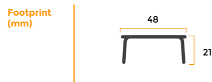
Closing profile for use when the flyscreen installation is not to be completed
