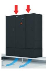
Execution for perimeter installation inside Data Centre. In this case, the sub-base side closure panels must be installed above the flooring. It is in any case essential to make sure that the height of the ceiling allows good air intake.
