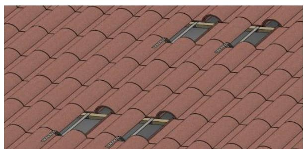
2.9. Fasten the structure to the 4 perforated steel strips (7) using 4 bolts, 4 nuts, and 4 washers.
