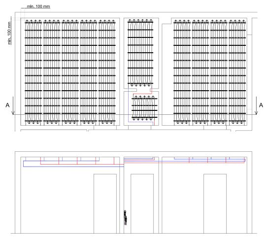
Fig. 1 Example of distribution for WW-10 ceiling panels
