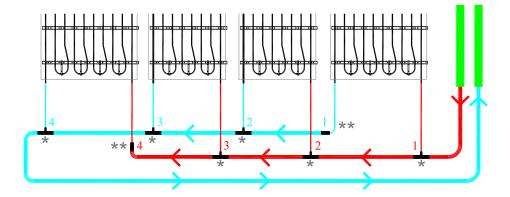
\* Mixed press-fit, push-fit Tee 10 -16 -10 mm
