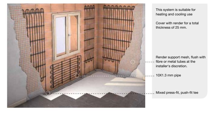
The WW-10 radiant system is very simple, made of radiant panels built starting with a 10 mm Ø pipe laid out to form a coil using suitable fixing bars and support brackets. The brackets are then fixed to the wall using hot glue or screws that are suitable for the base. These panels can be prefabricated, rather than built on site.
