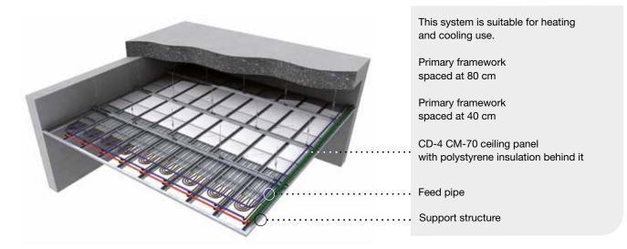
The CD-4 ceiling system is an innovative radiant heating and cooling system presented by WAVIN.
