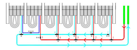
\* Mixed press-fit, push-fit Tee 10 -16 -10 mm
