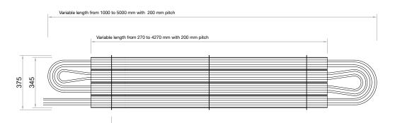
Metal supports for attaching to the structure, their number varies depending on the length of the panel
