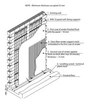
Sectional view of a wall radiant system, for structures made using premixed render, on a masonry support, and tile or marble cladding.
