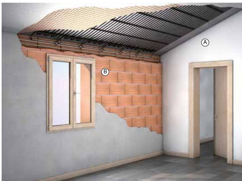
This system is suitable for heating and cooling use
