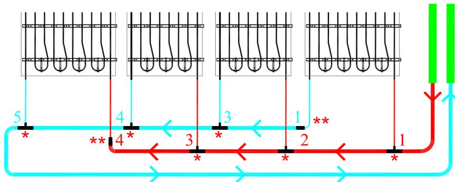
\* Mixed press-fit, push-fit tee 10 -16 -10 mm
