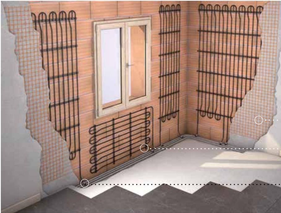
This system is suitable for heating and cooling use
