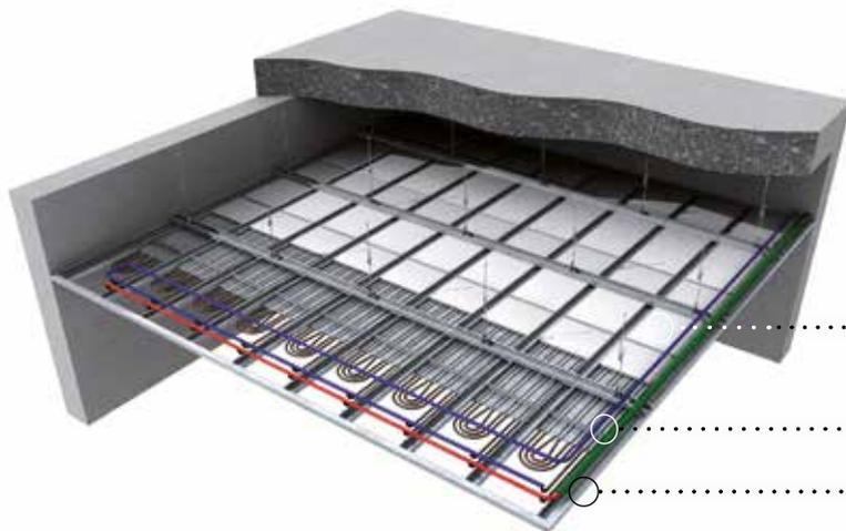
This system is suitable for heating and cooling use.
