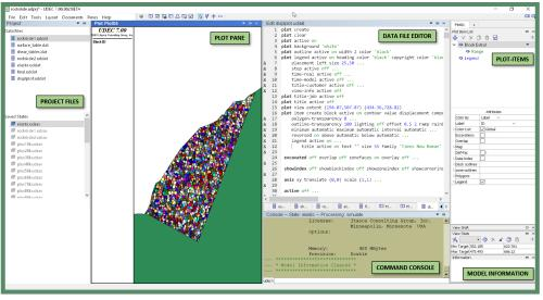
▲ The new, optional UDEC 7 graphical user interface provides pre- and post-processing tools, model analysis functionality, advanced plotting capabilities, file management tools, and a built-in data file editor. Multiple preset layouts are available; custom layouts may be saved. The familiar UDEC GIIC, with interactive modeling tools and project tree, is also available if preferred.
