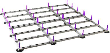
2) After having squared the entire structure and found the design of the flooring you can proceed to the fixing of the structures. Fix the substructures to each other at all intersections.
