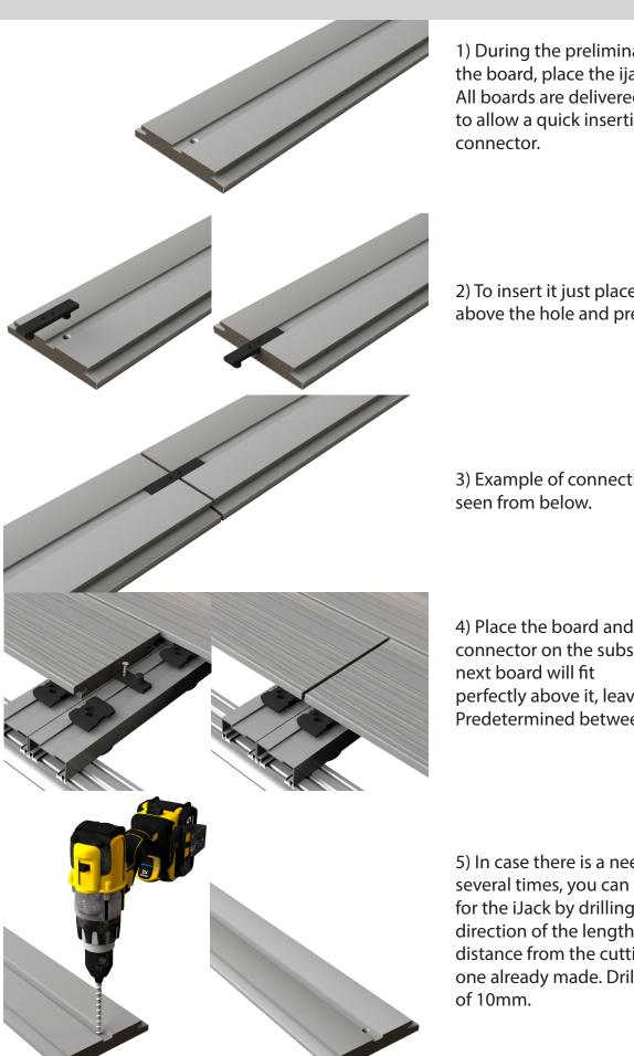
1) During the preliminary installation of the board, place the ijacks. All boards are delivered perforated to allow a quick inserting of the ljack
