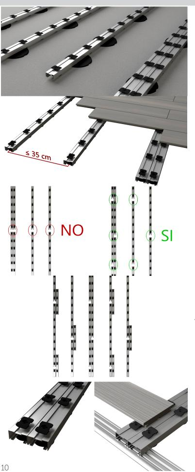
1) Place the **secondary substructure** with clips at a maximum distance of 35 cm. The secondary substructure can be fixed both to the existing base (flooring or screed) and to the primary substructure. N.B. use the 3-8mm regulator discs under the secondary structure if it is to be fixed directly to the base below.
