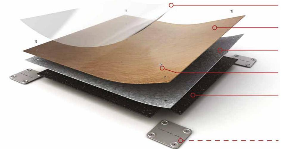
**SM02 Evolution** is a technical floor with a dry laying system. This is done by means of a support and mechanical coupling between tile and tile.
