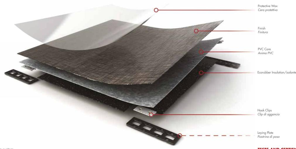
**PLO1 Invisible** is a technical floor with a dry laying system. This is done by one-click coupling between tiles.
