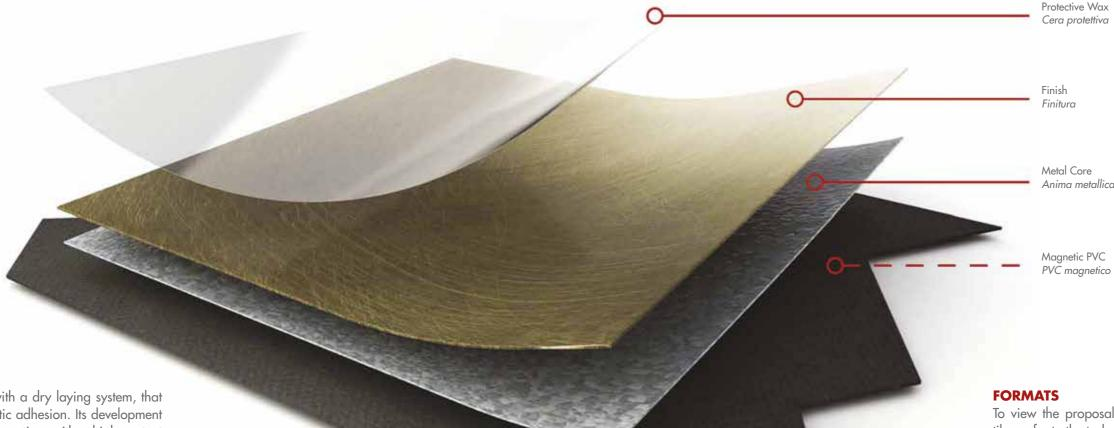
**MGO1 Magnetic** is a floor with a dry laying system, that can be installed through magnetic adhesion. Its development has followed criteria of new conception, with a high content of technology and design, with particular attention to the functionality and quality of the materials used, according to the criteria of the "Sustainable Project", to guarantee well-being and attention to the environment.
